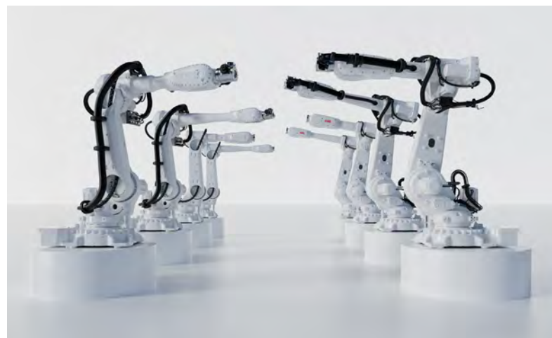
— IRB 5710, IRB 5720 large robots for material handling
