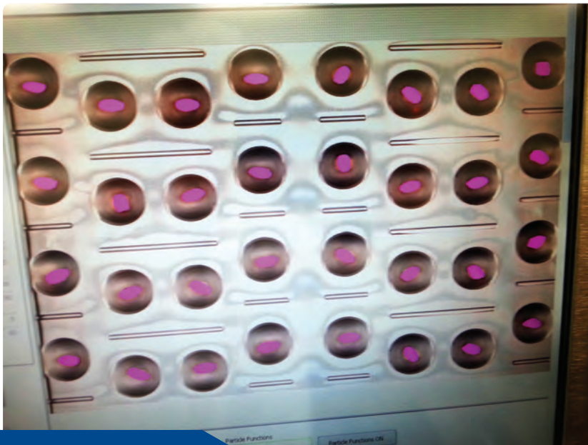
A setup screen of PCI's vision system looks at gel caps that are very light pink and nearly transparent. The pink areas show that the system is easily detecting gel caps with no background noise.
