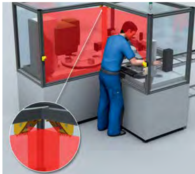
In this arrangement it is not possible to remain in the hazard zone without being detected. Therefore, a separate reset of the protective device is not necessary.
