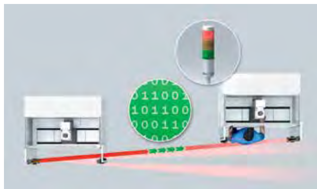
No mutual interference of protective devices due to the use of light beam coding – person is reliably detected and the hazardous movement is stopped.
