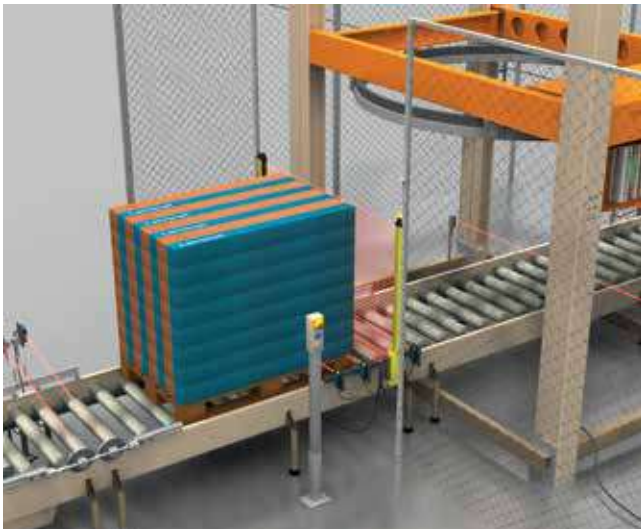
Muting function with safety light curtain and muting sensors on a wrapping machine.
