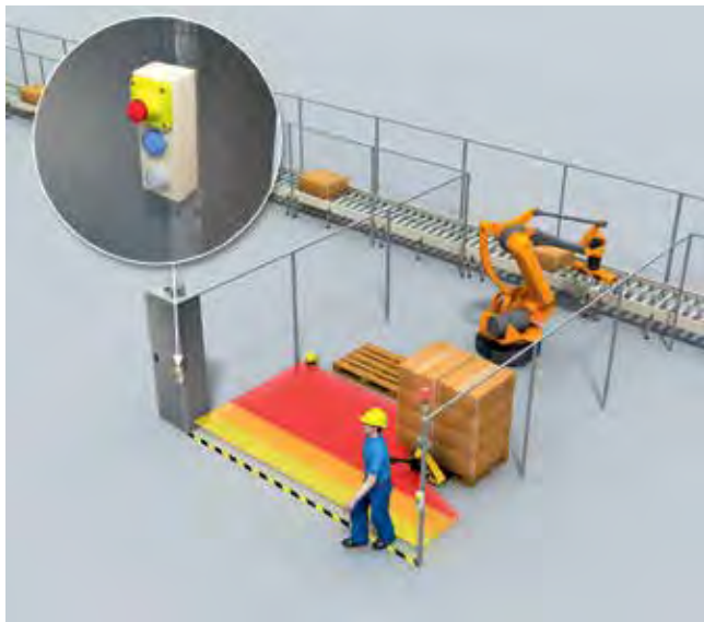
The position of the reset pushbutton allows a full view of the hazard zone for the resetting of the protective device.
