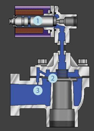
Contaminated Air Passes Through Unbalanced Solenoid Diaphragm Ruptures (Air Leaks) Small Fixed Orifice (Blocked By Contaminants) No Manual Override
