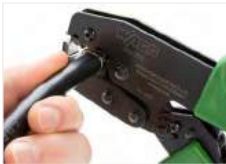
Squeeze handles until ratchet mechanism is released.
