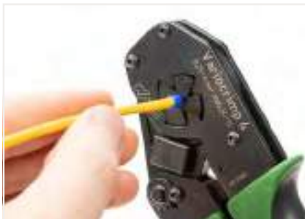
Squeeze handles until ratchet mechanism is released.
