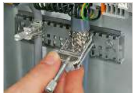
To remove the clamping saddle, unscrew until ratcheted mechanism is released, then slightly tip saddle and remove the clamping saddle.
