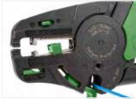
Cutting a conductor.
